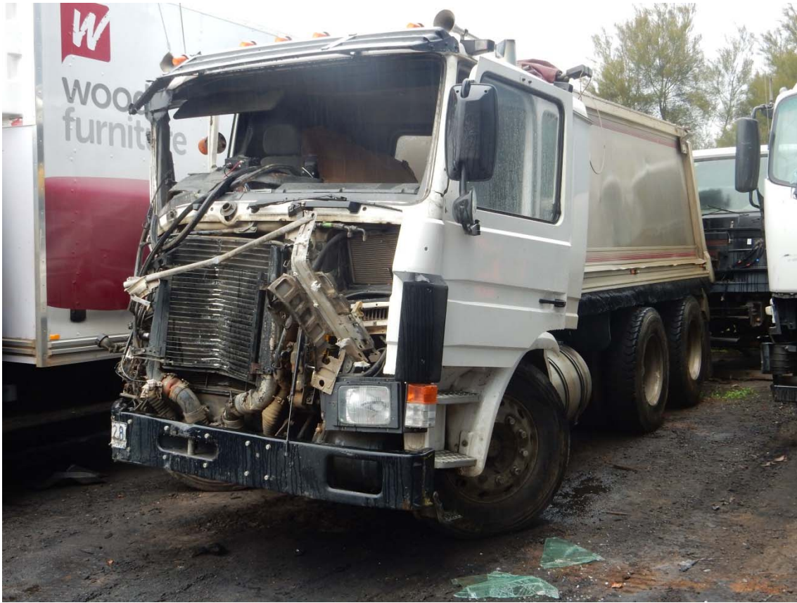
Figure 7: Collision damage to truck
